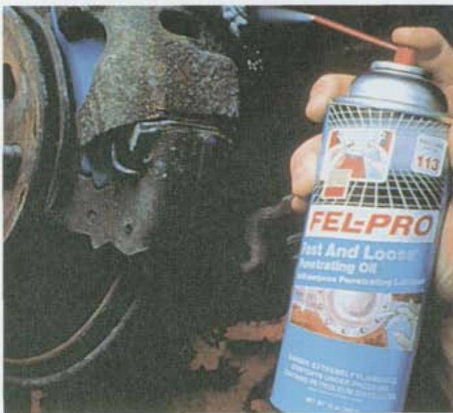
**Figure 9-21.** On rusted threads, such as those on this brake bleed screw, use rust penetrant to help ease turning and prevent breakage of the screw. (Fel-Pro Gaskets)
