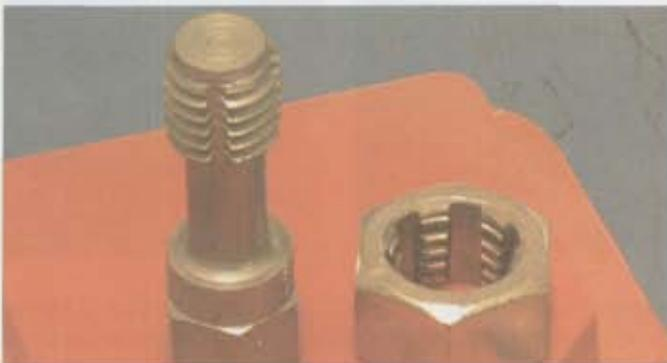
**Figure 9-14.** Thread chasers can be used to clean up slightly damaged internal or external threads. (Snap-on Tools)
