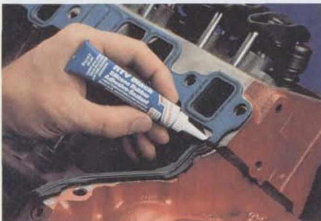
**Figure 9-25.** RTV sealer is commonly recommended where two different gaskets join. This sealer prevents leakage between the two gaskets.
