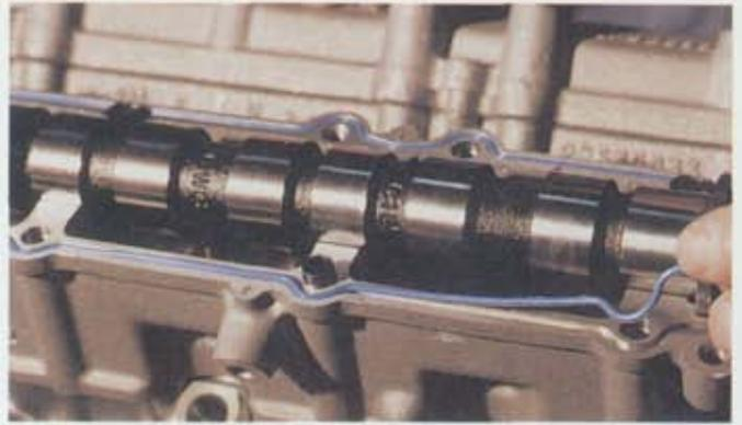
**Figure 9-30.** Many modern engines use synthetic seals instead of gaskets. This specially shaped seal fits down into a groove formed in the part.
